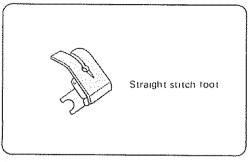
Use this foot exclusively for straight stitching using center needle position only.
